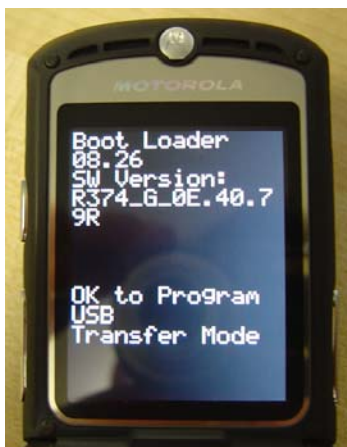
V3 in boot/flash mode (during stage 2 & 3 this may appear with out the writing)
